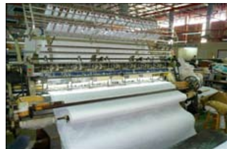
Polyester Batting being Quilted to the Outer Fabric on the Multi Quilting Machine
