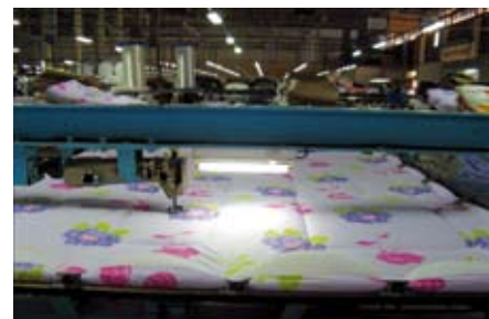
Quilting of Comforter being carried out on a Mechanised Quilting Machine
