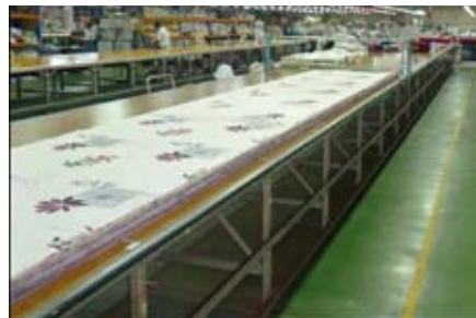
Cutting of Fabric from Bales on the Spreader Machine
